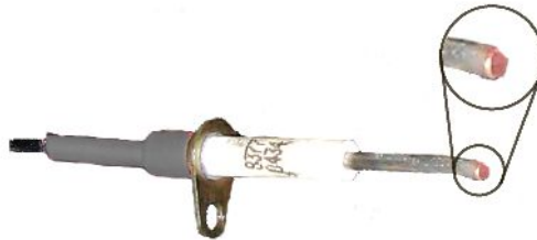
Figure 7: Spark Probe in Excellent Condition
